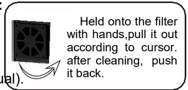
5. After using the machine for over 40 hours, please take off the dust filter and clean it (if have).
